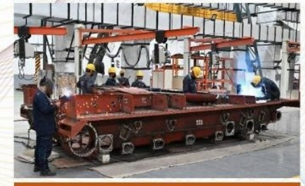
Welding of Armoured Plates - Tank Hull
