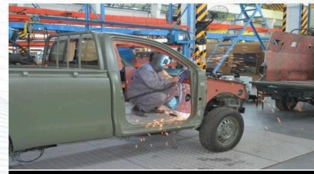
Production Line – Discrete Armouring Toyota Hilux
