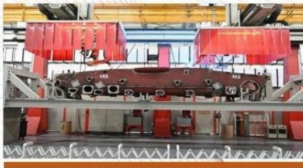
Robotic Arm Welding Station for Hull
